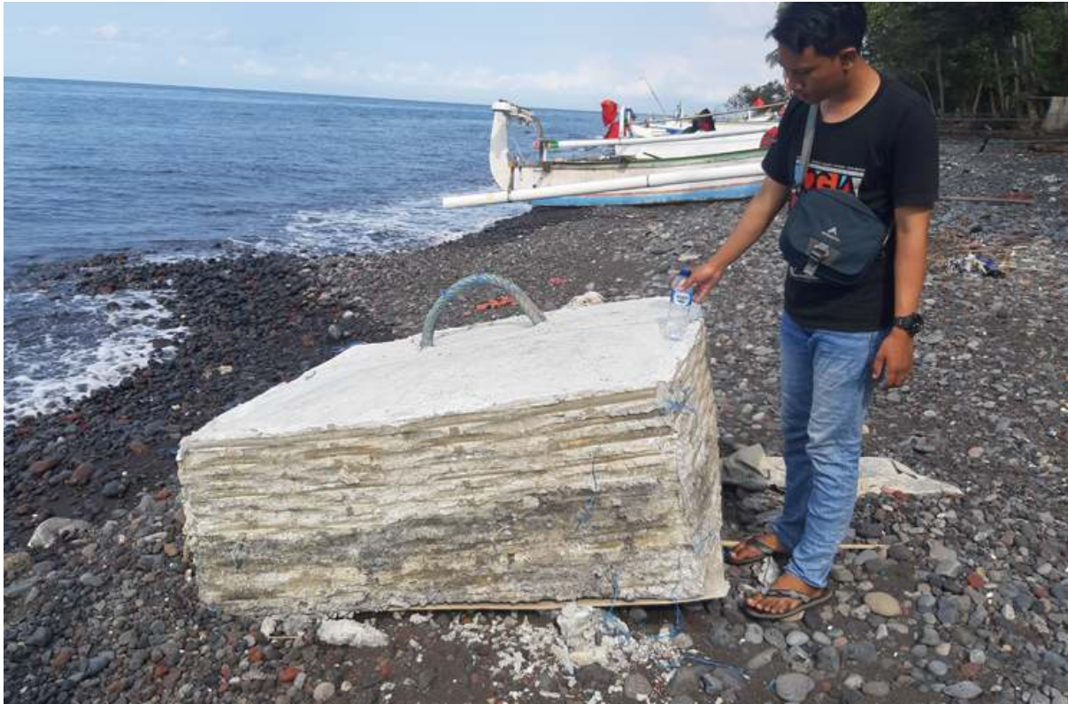
Figure 2.23: Cement concrete for anchoring FAD
