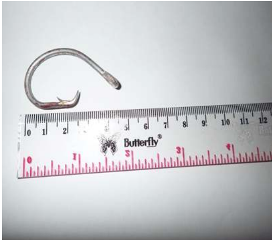
Figure 5.6: Typical C-hook used by weighted dropline single large hook targeting large tuna
